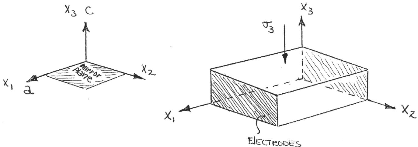
Your assignment is to determine the orientation, about  $x_3$ , in which surfaces should be ground on the crystal for application of the electrodes if the cell is to have optimum sensitivity.
