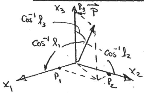
LET'S CONSIDER A VECTOR OF MAGNITUDE  $\|\vec{P}\|$  THAT IS DIRECTED IN A PARTICULAR ORIENTATION THAT WE CAN SPECIFY BY MEANS OF THE ANGLES  $\theta_1, \theta_2 \& \theta_3$  THAT IT MAKE WITH REFERENCE AXES  $x_1, x_2, x_3$
