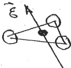
IN RESPONSE TO AN APPLIED ELECTRIC FIELD  $\vec{E}$ . THE PROPERTY RELATING THE TWO VECTORS IS THE ELECTRONIC POLARIZABILITY  $\alpha$
