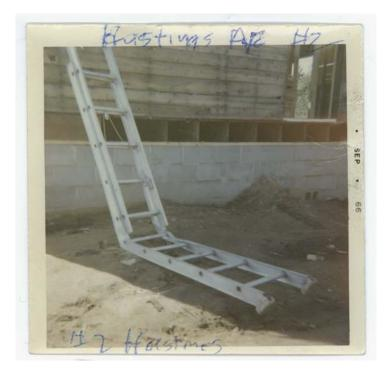
Figure 2: Failed aluminum ladder.
