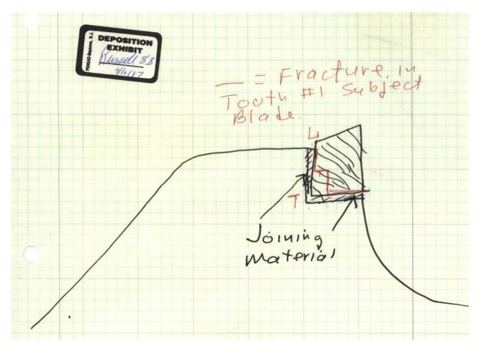
Figure 1: Schematic of saw blade, showing how the carbide tooth fractured both along the join and through the carbide.
