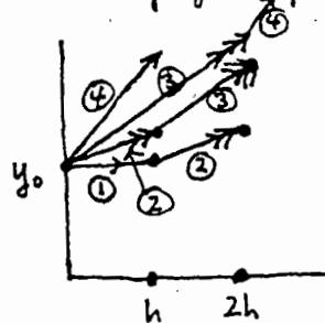
We calculate, in R-K method, the 4 slopes marked  $\textcircled{1} \rightarrow \textcircled{4}$
