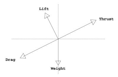
FIGURE 1. Forces on an airfoil
