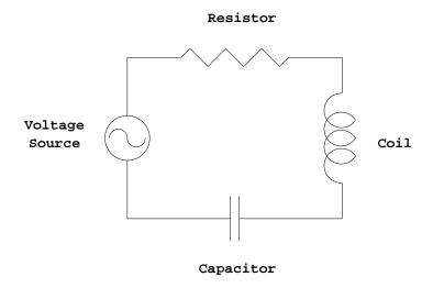
FIGURE 5. Series RLC Circuit
