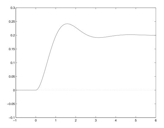
FIGURE 14. The unit step response for  $\ddot{x} + 2\dot{x} + 5x$
