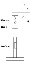
Figure 6. Spring-driven system
