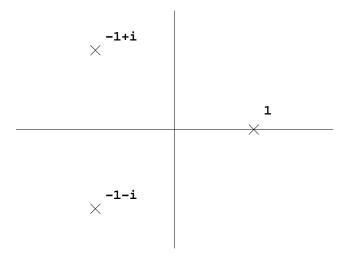
FIGURE 15. Pole diagram for  $1/(s^3 + s^2 - 2)$
