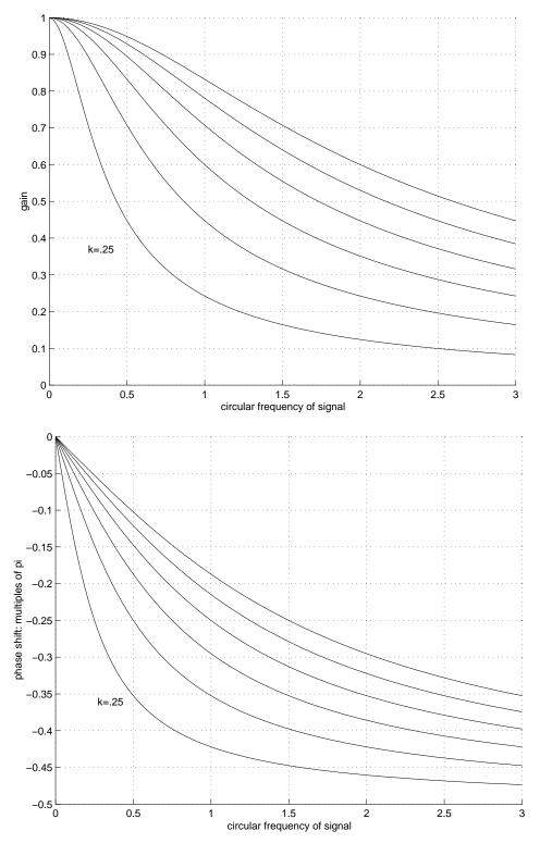
FIGURE 2. First order amplitude response curves
