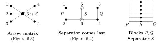
Figure 6.6: A graph separator numbered last produces a block arrow matrix K.
