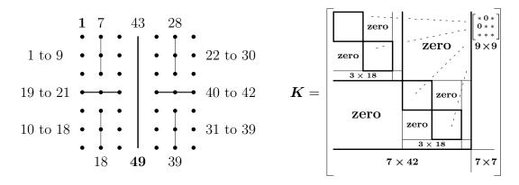
Figure 6.7: Three levels of separators. Still  $\underline{\hspace{1cm}}$  nonzeros in K, only  $\underline{\hspace{1cm}}$  in L.
