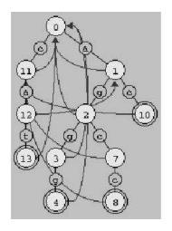
Figure 10.4: A multiple pattern FSM.
