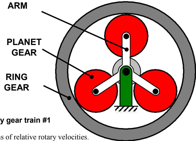
Example:  $N_{s1}$  = Number of teeth on sun gear in planetary gear train #1
