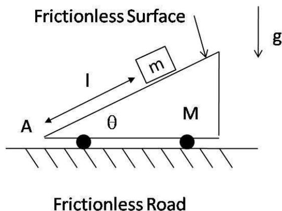
Figure 4: Block on frictionless surface that moves on frictionless road. The mass ( $m$ ) can slide down the incline in a frictionless manner. Mass ( $M$ ) is free to move horizontally without friction. If mass ( $m$ ) is released from rest at the  $l$  position, find the velocity of mass ( $M$ ) at the moment ( $m$ ) reaches the bottom of the incline. Figure by MIT OCW.
