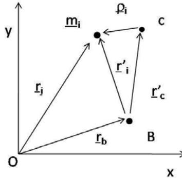
Figure 1: Angular momentum about  $B$  for a system of particles. Each particle has mass  $m_i$  positions  $r_i$  with respect to the origin and  $r'_i$  with respect to  $B$ . The center of mass  $C$  has positions  $r'_c$  with respect to  $B$  and  $\rho_i$  with respect to each point mass  $m_i$ . Figure by MIT OCW.
