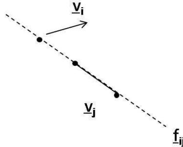
Figure 2: Relative velocity probably has a component in the direction of  $\underline{f}_{ij}$ . The figure shows two random points with randomly chosen velocities. Unless the difference between the velocities of the two points is zero or perpendicular to the direction of force  $\underline{f}_{ij}$ ,  $\underline{f}_{ij} \cdot (\underline{v}_i - \underline{v}_j)$  will not be zero; there would be some component in the direction of  $\underline{f}_{ij}$ . Figure by MIT OCW.
