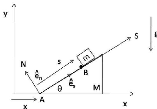
Figure 5: Diagram of kinematics of block on ramp. Need two sets of coordinates.  $M$  only moves in the  $x$ -direction.  $m$  only moves in the  $\hat{e}_s$  direction. Figure by MIT OCW.
