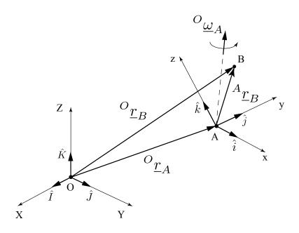
$${}^{O}\underline{V}_{B} = {}^{O}\underline{V}_{A} + {}^{A}\underline{V}_{B}|_{O\underline{\omega}_{A}=0} + {}^{O}\underline{\omega}_{A} \times {}^{A}\underline{r}_{B}$$
