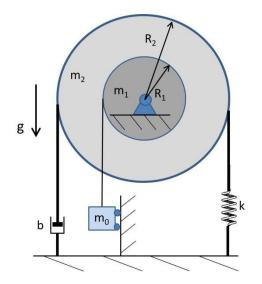
wrapped without slipping around the larger cylinder. The two ends of the string are connected to a spring of constant k on one end and a dashpot of constant b at the other. The smaller cylinder is connected to a block of mass m<sub>o</sub> via an inextensible massless strap, which is wrapped without slipping around the smaller cylinder. The block is constrained to move only vertically.
