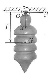
figure. The center of mass is at a distance 'l' from O and  $I_{zz/G}$  is known. An external time varying torque,  $\tau(t)$  is applied to the pendulum at O.
