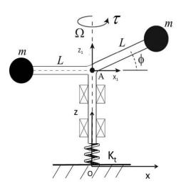
vertical shaft. The shaft rotates with a time varying angular velocity  $\Omega$  with respect to the  $O_{xyz}$  inertial frame. The arms are of length L. The frame  $A_{xlylzl}$  rotates with the arms and attached masses. A time varying torque is applied to the rotor about the z axis, such that  $\tau_{/A} = \tau_o(t) \hat{k}$ . Note that the angle  $\phi$  is fixed.
