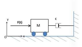
a). Use Lagrange's equations to derive the equation(s) of motion for the system.
