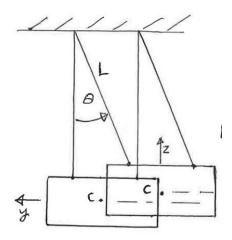
damping. After 5 cycles of vibration the maximum angle of motion has reduced to 0.08 radians. What is the approximate damping ratio of the system.
