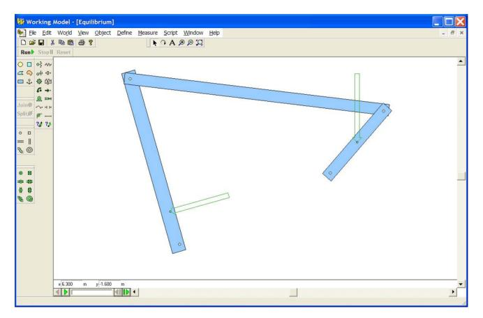
• If the only forces on a body act through 2 pin joints, then the net force acts along the line between the 2 joints.
