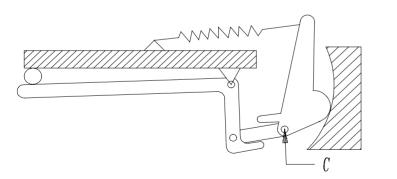
VMA II MECHANISM STOP FOR COUPLER SWITCHED TO OTHER SIDE
