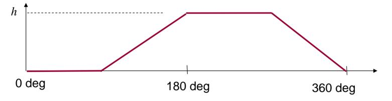
Sketch the velocity and acceleration curves  The following <u>acceleration</u> curve is proposed for a cam device
