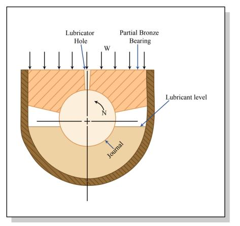
Say a railroad tank car creates the downward force *W*. The projected area of the partial bearing was *A*. Tower observed that the gauge pressure measured from the "lubricator hole" was about *2W/A*.
