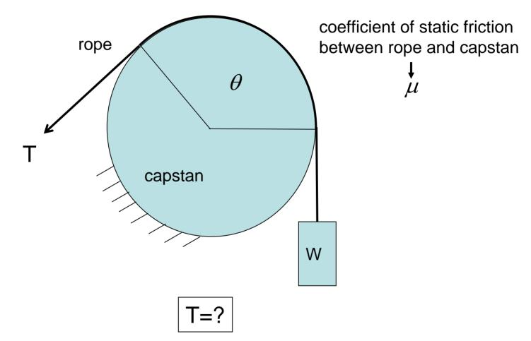
What is the smallest value of T that will keep the weight W from beginning to move downward?
