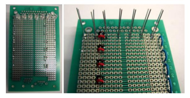
Figure 8: First Row of LEDs: Back (Left) and Front (Right)
