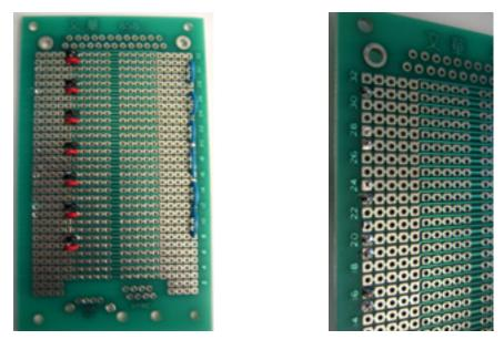
Figure 7: Protoboard with Row Connection Wires: Front (left) and Back (right)
