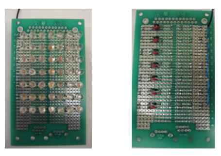
Figure 11: All Rows of LEDs: Back (Left) and Front (Right)
