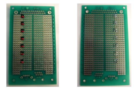
Figure 6: Protoboard with Jump Wires: Front (left) and Back (right)
