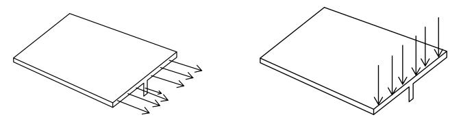
in the second case the axial stress is transmitted to the outer fibers of the flange by shear if the stress were transmitted without deformation (strain) there would be no difference but ..... that is not the case. There will be less stress at the ends of the flange and more at the web.
