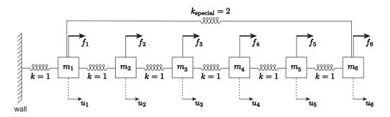
Figure 2: The spring-mass system for Question 3. Note that all the spring constants are unity, k = 1, except for the "special" spring which links mass 1 and mass 6,  $k_{\text{special}} = 2$ . Note that all the springs are described by the linear Hooke relation.
