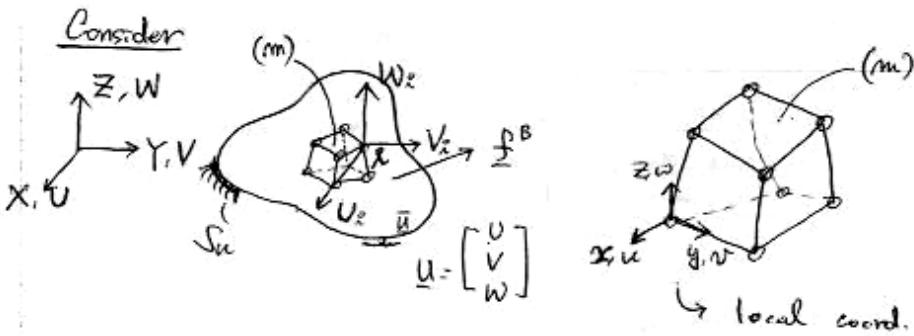
$$\hat{\mathbf{U}}^T = [ U_1 \quad V_1 \quad W_1 \quad U_2 \quad \dots \quad W_N ] \quad (N \text{ nodes}) \quad (4.4)$$
