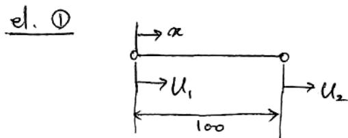
$$u^{(1)}(x) = \underbrace{\begin{bmatrix} 1 - \frac{x}{100} & \frac{x}{100} & 0 \end{bmatrix}}_{H^{(1)}} \begin{bmatrix} U_1 \\ U_2 \\ U_3 \end{bmatrix} \quad (4.19)$$
