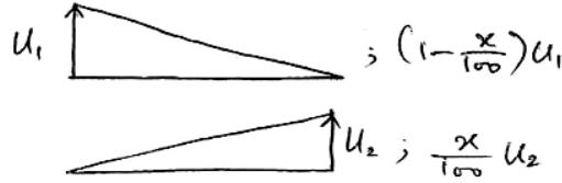
$$\epsilon_{xx}^{(1)}(x) = \underbrace{\begin{bmatrix} -\frac{1}{100} & \frac{1}{100} & 0 \end{bmatrix}}_{B^{(1)}} \begin{bmatrix} U_1 \\ U_2 \\ U_3 \end{bmatrix} \quad (4.20)$$
