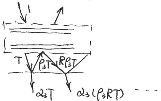
The effective absorptance of the solar collector is:
