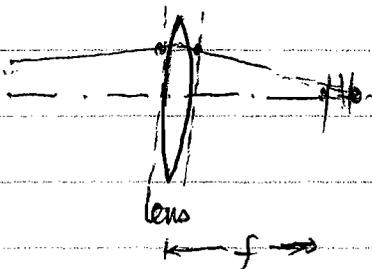
$$\begin{pmatrix} w_{out} \\ w'_{out} \end{pmatrix} = \begin{pmatrix} 1 & 0 \\ -1/f & 1 \end{pmatrix} \begin{pmatrix} w_{in} \\ w'_{in} \end{pmatrix}$$
