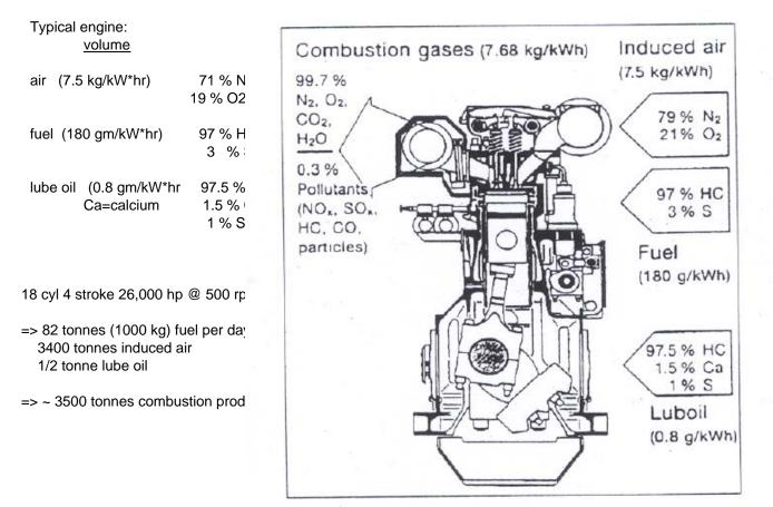
Fig. 3 Specific mass flow rates of a large medium-speed diesel engine
