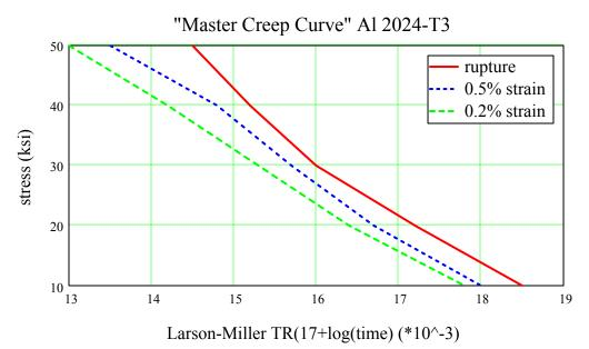
The Larson Miller parameter combines temperature and times (rupture, strain) as follows:
