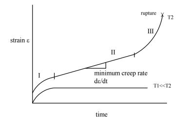
stage I: primary creep: rapid initial deformation stage II: secondary creep: a.k.a. steady state creep: constant strain rate designated "minimum strain rate"
