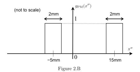
2. Spatial filtering Figure 2.A above shows a 4F imaging system with two identical lenses L1, L2 of focal length f = 5cm. The illumination wavelength is  $\lambda = 1\mu$ m. The transmissivity of the pupil mask is shown in Figure 2.B.
