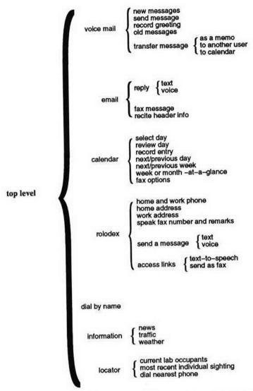
Figure 12.12. Phoneshell's menus provide access to a variety of personal information management functions.
