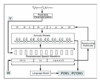
Figure 5. This diagram from Young (1996) shows the computation of the probability P(WIY) of word sequence W given the parameterized acoustic signal Y. The prior probability P(W) is determined directly from a language model. The likelihood of the acoustic data P(YIW) is computed using a composite hidden Markov model representing W constructed from simple HMM phone models joined in sequence according to word pronunciations stored in a dictionary.
