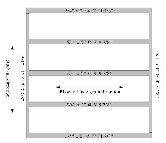
Figure 1: Frame construction layout
