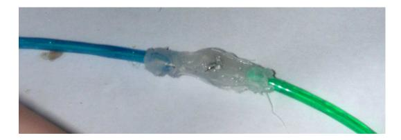
Figure 8: EL wire connection — glued
