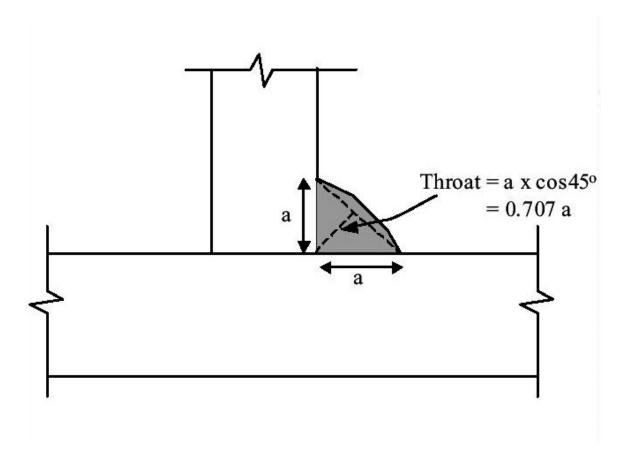
The strength of the weld to resist shearing force is the product of ¾ times half the square root of two times the distance "a" marked above times the length of the weld, times the shear strength of the weld material, often comparable to the shear strength of the steel. The final part appear below:
