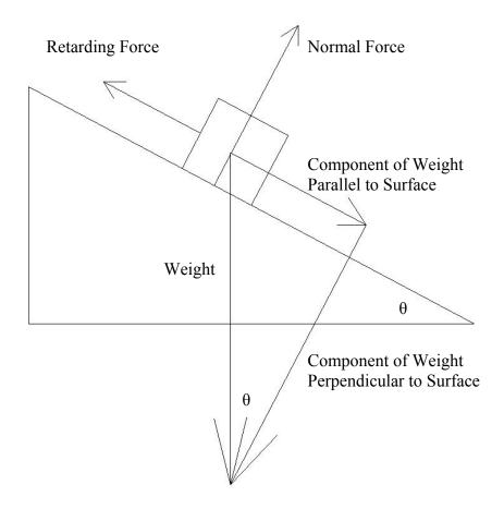
There are three main forces acting on the turntable, represented above as the block, on the inclined plane of the rake stage, which is at an angle  $\theta$  above the horizontal. The first is the weight of the block, which, due to gravity, pulls straight downwards. The second is the normal force of the stage supporting the turntable, perpendicular to the
