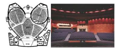
This is a schematic and a picture of a theater in Edinburgh, Scottland, which features two massive turntables with raked tops, in this case holding seats. By rotating the seating sections, the theater can become one massive conglomerate, or one medium sized auditorium and two mini auditoriums. While innovative, this application is not one where the turntable itself is raked; rather, the structure on top is raked.
