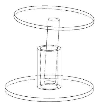
Now, instead of being able to move freely, the pivot is likely to bind in its movement, with the entirety of the force being applied at two points, causing immense friction at those two small places, in addition to deformation of the material with would enhance the friction. Also, since these plates are fairly small relative the forces involved, it might be possible that they would rip out of either the turntable or off the stage, causing catastrophic failure. Thus this design is not sufficient
