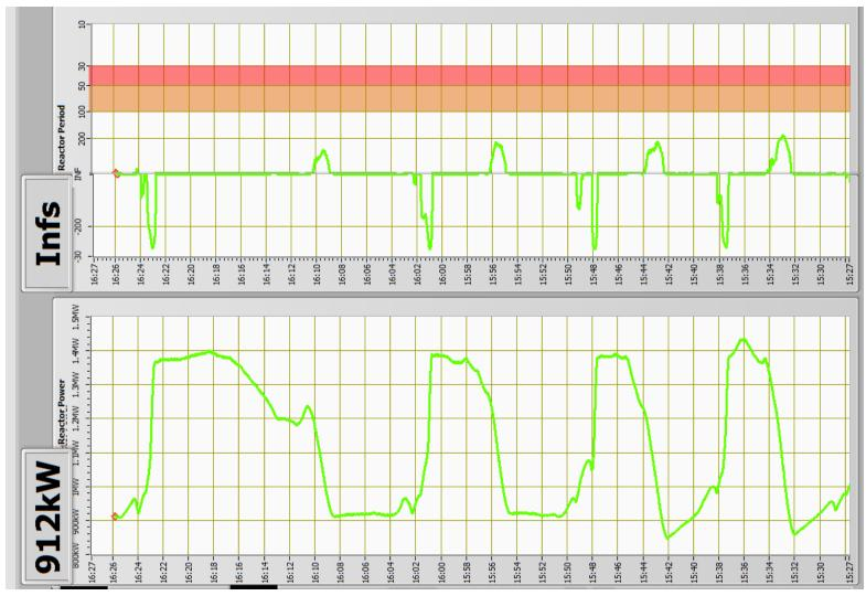
The graph on the bottom is the reactor power, while the graph on top is the "reactor period," which is the mean time that it would take for the reactor to increase in power by a factor of e. There are a few features to notice here:
