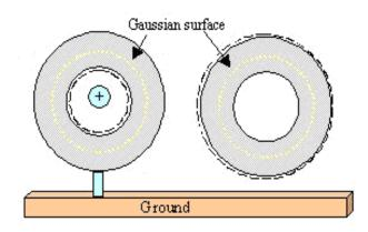
Figure 2 Grounding the ice pail (left) and after removing the ground & ball (right)
