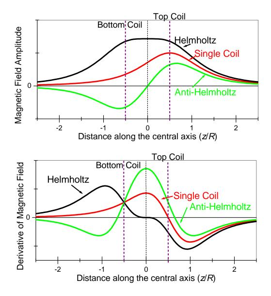
**Figure 2:** The *z*-component of the magnetic field and its derivative for the three modes of operation of the Helmholtz coil. See page the last page of this write-up for an "iron-filings" representation of these three field configurations.
