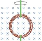
In each of the cases pictured above, the magnetic flux into the page is decreasing with time (because the (1) B field, (2) loop area or (3) projected area are decreasing with time). This decreasing flux creates an EMF. In which direction? We can use Lenz's Law to find out.
