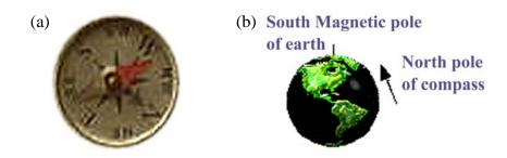
**Figure 1** (a) A mini-compass like the ones we will be using in this lab. (b) The painted end of the compass points north because it points towards magnetic south.
