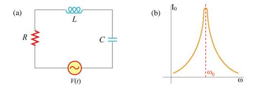
Figure 3 Driven *RLC* Circuit. (a) The circuit (b) The magnitude of the oscillating current  $I_0$  reaches a maximum when the circuit is driven at its resonant frequency
