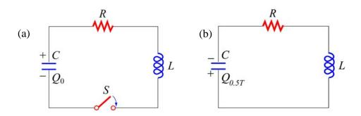
**Figure 2 Undriven RLC circuit.** (a) For t<0 the switch S is open and although the capacitor is charged  $(Q = Q_0)$  no current flows in the circuit. (b) A half period after closing the switch the capacitor again comes to a maximum charge, this time with the positive charge on the lower plate.
