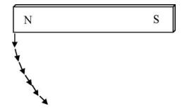
4. Repeat the process described above several more times (~4 field lines), starting at different locations on the magnet. Work fairly quickly – it is more important to get a feeling for the shape of the field lines than to map them precisely.
