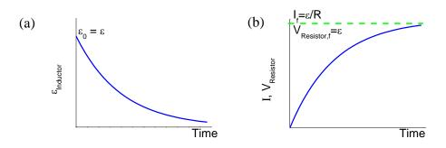
**Figure 6** (a) "EMF generated by the inductor" decreases with time (this is what a voltmeter hooked in parallel with the inductor would show) (b) the current and hence the voltage across the resistor increase with time, as the inductor 'relaxes.'
