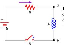
**Figure 5 RL circuit.** For t<0 the switch S is open and no current flows in the circuit. At t=0 the switch is closed and current *I* can begin to flow, as indicated by the arrow.
