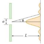
The next kind of interference we consider is light going through a single slit, interfering with itself. This is called diffraction, and arises from the finite width of the slit (*a* in the picture at left). The resultant effect is not nearly as easy to derive as that from two-slit interference (which, as you can see from above, is straightforward). The result for the anglular locations of the minima is  $a \sin(\theta) = m\lambda$ .
