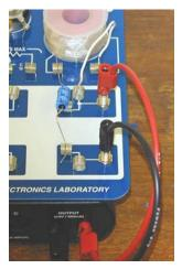
We will also again use the circuit board, set up with a 100  $\mu$ F capacitor in series with the coil (which serves both as the resistor and inductor in the circuit), as pictured at left.
