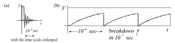
Figure 2 Charging and Discharging the Capacitor. The capacitor is slowly charged (limited by the RC time constant, with  $R = 4.5 M\Omega$ ) and then (a) rapidly discharges across the spark gap, resulting in (b) a series of slow charge/rapid discharge bursts. This is an example of a "relaxation oscillator."
