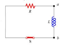
After a long time *T* the current will reach an equilibrium value and inductor will be "fully charged." At this point we turn off the battery ( $\varepsilon$ =0), allowing the inductor to 'discharge,' as pictured at left. Repeat each of the steps a-c in problem 4, noting that instead of  $\exp(-t/\tau)$ , our expression for current will now contain  $\exp(-(t-T)/\tau)$ .
