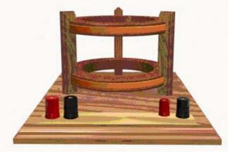
Figure 3 Helmholtz Coil Apparatus
