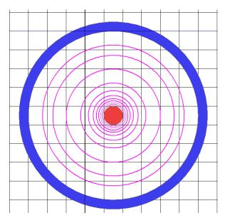
One group did this lab and measured the equipotentials for a slightly different potential landscape then the ones you have been given (although still on a 1 cm grid) and using +10 V rather than +5V.
