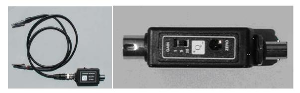
**Figure 5** Charge Sensor – measures voltage difference between its red and black leads. Left: Shown attached to the lead assembly. Right: The gain switch (used to amplify small signals) should be set at 1. The zero button sets the output signal to zero.
