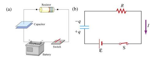
**Figure 2** (a) *RC* circuit (b) Circuit diagram for t > 0
