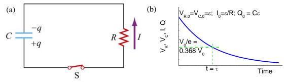
**Figure 4** Once (a) the battery is "turned off," the voltages across the capacitor and resistor, and hence the charge on the capacitor and current in the circuit all (b) decay exponentially. The time constant  $\tau$  is how long it takes for a value to drop by e.
