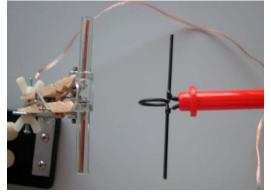
These have been described in detail above. The spark gap of the transmitter (pictured left) can be adjusted by turning the plastic wing nut (top). It is permanently wired in to the high voltage power supply on the circuit board. The receiver (pictured right) must be plugged in to the circuit board.
