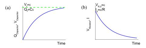
**Figure 3** (a) Voltage across and charge on the capacitor increase as a function of time while (b) the voltage across the resistor and hence current in the circuit decrease.
