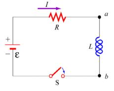
Consider the circuit at left, consisting of a battery (emf  $\varepsilon$ ), an inductor *L*, resistor *R* and switch *S*.
