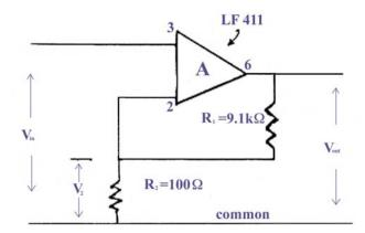
a) What is the output voltage  $V_{out}$  of the op-amp in terms of the input voltage  $V_{in}$  to pin 3, and the voltage at pin 2,  $V_2$ , and the amplification A? (Note: all voltages are with respect to common).
