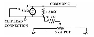
a) When the  $5k\Omega$  pot is turned 2/3 of the way in the direction of the +6V line from the -6V end, what is the voltage difference between common C and the  $5k\Omega$  pot slider?
