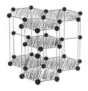
In each plane the atoms are at the corners of open hexagons. The odd-numbered layers are all identical when viewed from above. All even-numbered layers are also identical, but they are shifted with respect to the odd layers. Describe this structure by giving the lattice type, the primitive unit cell, and the basis.
