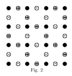
(b) In LaCuO one discovers, at closer inspection, that the copper oxide lattice is actually not flat, but that the oxygen atoms are moved a small amount out of the plane ("up" or "down") in an alternating fashion (see Fig. 2. a + means up and a - means down) What is the primitive cell and lattice spacing for this crystal? What is the basis?
