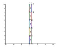
Figure 3: Geometry of a tower with 5 segments with labeled nodes.
