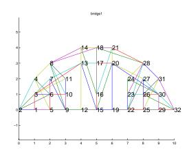
Figure 1: Geometry of a bridge1 with labeled nodes.
