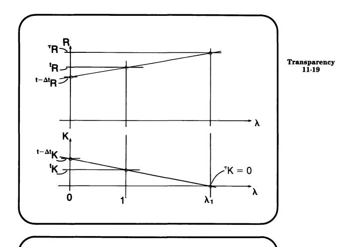
The problem of solving for  $\lambda$  such that  $det(\underline{K}) = 0$  is equivalent to the eigenproblem
