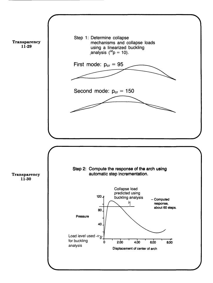
We have computed the response of a perfect (symmetric) arch. Because the first collapse mode is antisymmetric, that mode is not excited by the pressure loading during the response calculations.
