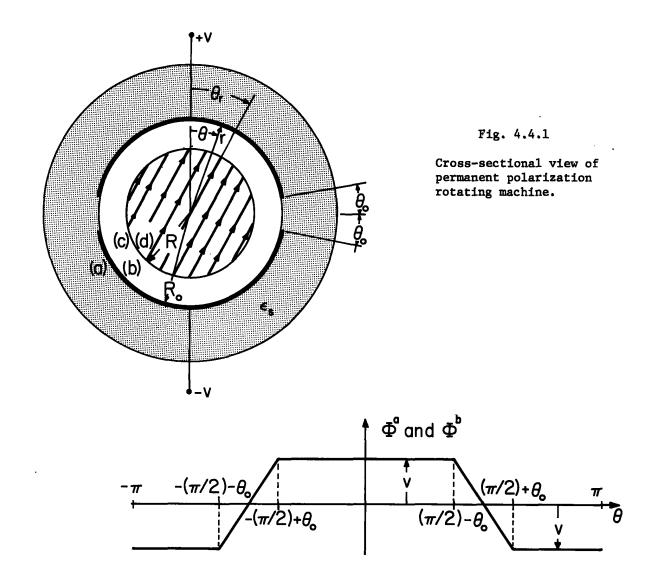
Fig. 4.4.2. Distribution of stator potential used to model the device shown in Fig. 4.4.1.
