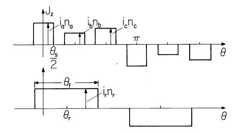
Fig. 4.9.3 Azimuthal current density distribution on stator and rotor.
