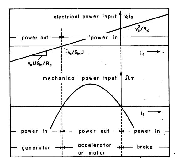
Fig. 4.10.5. Regimes of energy conversion for a d-c magnetic field type interaction. Armature voltage  $v_a$  is fixed and field current  $i_f$  is varied. With the identification of variables  $i_f \rightarrow v_f$ ,  $v_a \rightarrow i_a$ ,  $R_a \rightarrow R_a^{-1}$ ,  $G_m \rightarrow G_e$ , the power characteristics also represent the Van de Graaff type of device developed in Sec. 4.14.
