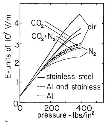
Fig. 4.15.2. Breakdown strength of common gases as a function of gas pressure for several different electrode combinations.<sup>2</sup>
