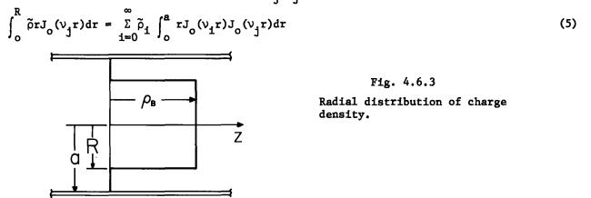
The right-hand side is integrated using Eq. 4.5.32, while the left-hand side is an integral that can be evaluated from tables or by using the fact that  $J_0(v_1r)$  satisfies Eq. 4.5.20 with m = 0 and Eq. 2.16.26c holds for  $J_{a}$ :
