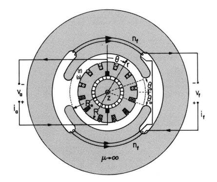
Fig. 4.10.1. Cross section of d-c machine.
