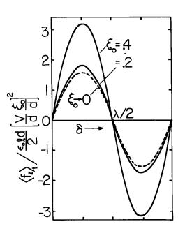
Fig. 4.13.2a. Electrical force on rotor of variablecapacitance machine (Fig. 4.12.1) as a function of normalized relative displacement  $\underline{z}_r = z_r/\lambda$ , with amplitude of electrodes as a parameter.
