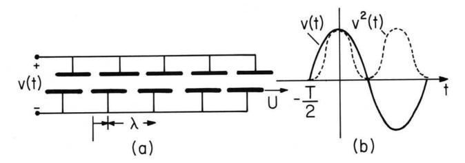
Fig. 4.13.1. Physical realization of variable-capacitance machine modeled in Fig. 4.12.1.
