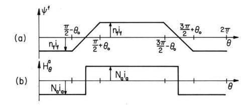
Fig. 4.10.2. Circumferential distribution of magnetic potential at r = Rand tangential magnetic field intensity at r = R.
