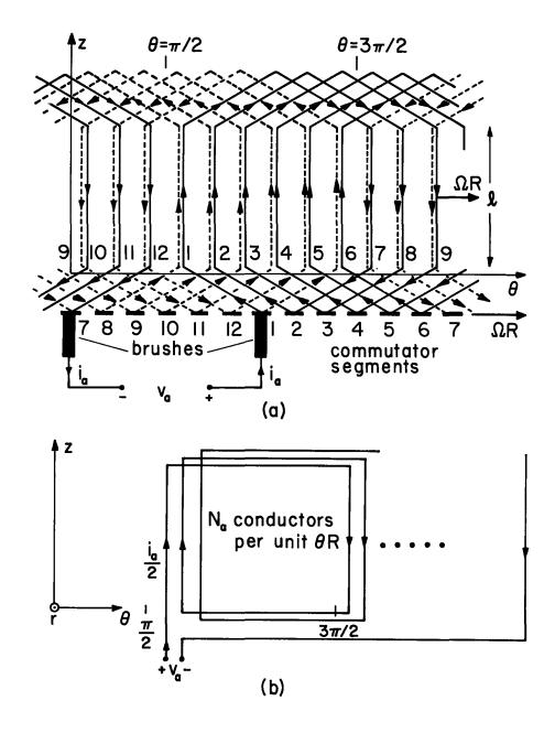
Fig. 4.10.3. (a) Typical winding scheme for armature of d-c machine shown in Fig. 4.10.1. The r axis is directed out of the paper. Brushes make contact with commutator segments which move to the right with armature conductors.<sup>2</sup> (b) Winding distribution of solid wires.
