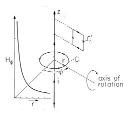
Fig. 1.4.4 Uniform line current with contours for determining H. Axis of rotation is used to deduce that radial component of field must be zero.
