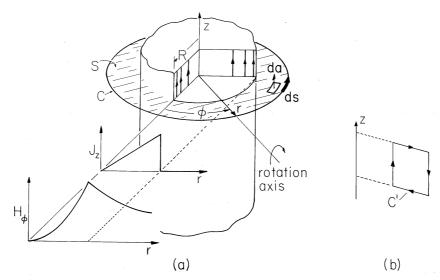
**Fig. 1.4.2** Axially symmetric current distribution and associated radial distribution of azimuthal magnetic field intensity. Contour C is used to determine azimuthal  $\mathbf{H}$ , while C' is used to show that the z-directed field must be uniform.
