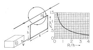
**Fig. 1.6.4** Demonstration of voltmeter reading induced at terminals of a coil in accordance with Faraday's law. To plot data on graph, normalize voltage to  $V_o$  as defined with (11). Because I is the peak current, v is the peak voltage.
