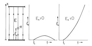
**Fig. 1.1.2** An electron, subject to the uniform electric field intensity  $\mathbf{E}_x$ , has the position  $\xi_x$ , shown as a function of time for positive and negative fields.
