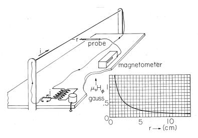
Fig. 1.4.5 Demonstration of peak magnetic flux density induced by line current of 6 ampere (peak).
