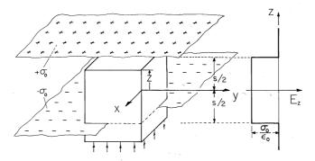
Fig. 1.3.8 Sheets of surface charge and volume of integration with upper surface at arbitrary position x. With field  $E_o$  due to external charges equal to zero, the distribution of electric field is the discontinuous function shown at right.
