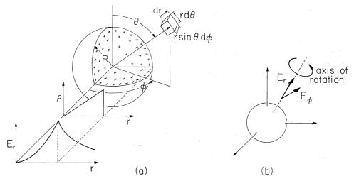
**Fig. 1.3.2** (a) Spherically symmetric charge distribution, showing radial dependence of charge density and associated radial electric field intensity. (b) Axis of rotation for demonstration that the components of **E** transverse to the radial coordinate are zero.
