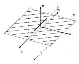
**Fig. 1.4.7** Ampère's integral law is applied to surface S' enclosed by a rectangular contour that intersects a surface S carrying the current density K. In terms of the unit normal to S, n, the resulting continuity condition is given by (16).
