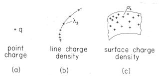
Fig. 1.3.3 Singular charge distributions: (a) point charge, (b) line charge, (c) surface charge.
