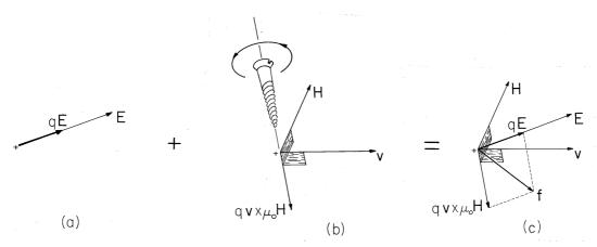
**Fig. 1.1.1** Lorentz force f in geometric relation to the electric and magnetic field intensities, E and H, and the charge velocity v: (a) electric force, (b) magnetic force, and (c) total force.
