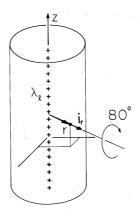
Fig. 1.3.7 Uniform line charge distributed from - infinity to + infinity along z axis. Rotation by 180 degrees about axis shown leads to conclusion that electric field is radial.
