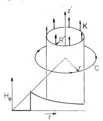
**Fig. 1.4.6** Uniform current density  $K_o$  is z directed in circular cylindrical shell at r = R. Radially discontinuous azimuthal field shown is determined using the contour at arbitrary radius r.
