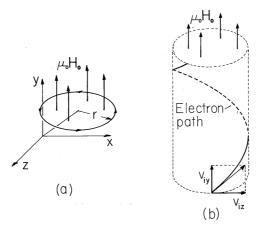
Fig. 1.1.3 (a) In a uniform magnetic flux density  $\mu_o \mathbf{H}_o$  and with no initial velocity in the y direction, an electron has a circular orbit. (b) With an initial velocity in the y direction, the orbit is helical.
