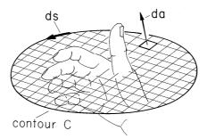
**Fig. 1.4.1** Surface S is enclosed by contour C having positive direction determined by the right-hand rule. With the fingers in the direction of  $d\mathbf{s}$ , the thumb passes through the surface in the direction of positive  $d\mathbf{a}$ .
