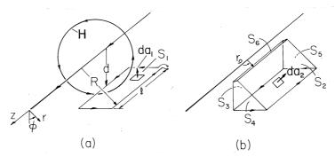
**Fig. 1.7.2** (a) The field of a line current induces a flux in a horizontal rectangular coil. (b) The open surface has the coil as an enclosing contour. Rather than being in the plane of the contour, this surface is composed of the five segments shown.
