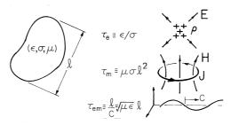
**Fig. 15.3.1** Arbitrary system having typical length l, permittivity  $\epsilon$ , conductivity  $\sigma$ , and permeability  $\mu$ .
