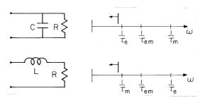
Fig. 15.4.1 Low-frequency equivalent circuits and associated ordering to reciprocal times.
