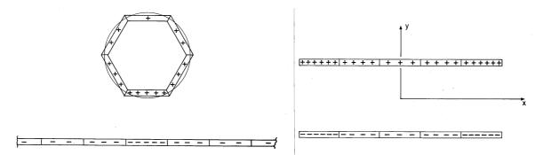
Fig. 4.8.1 (a) Surface of circular cylinder over a ground plane broken into planar segments, each having a uniform surface charge density. (b) Special case where boundaries are in planes y = constant.
