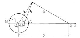
**Fig. 4.6.7** Cross-section of spherical electrode having radius R and center at the origin of x axis, showing charge q at x = X. Charge  $Q_1$  at x = D makes spherical surface an equipotential, while  $Q_o$  at origin makes the net charge on the sphere zero without disturbing the equipotential condition.
