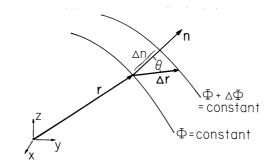
Fig. 4.1.2 Two equipotential surfaces shown cut by a plane containing their normal,  ${\bf n}.$
