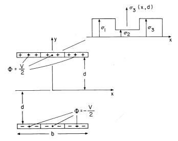
Fig. 4.8.3 Charge distribution on plane parallel electrodes approximated by six uniformly charged strips.
