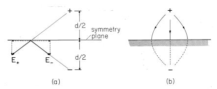
Fig. 4.7.1 (a) Field of positive charge tangential to horizontal plane is canceled by that of symmetrically located image charge of opposite sign. (b) Net field of charge and its image.
