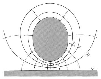
**Fig. 4.6.3** The  $\underline{\Phi} = 1$  and  $\underline{\Phi} = 0$  equipotentials of Fig. 4.5.6 are turned into perfectly conducting electrodes having the capacitance of (4.6.16).
