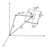
Fig. 4.5.2 An element of surface charge at the location  $\mathbf{r}'$  gives rise to a potential at the observer point  $\mathbf{r}.$
