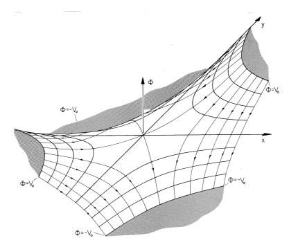
**Fig. 4.1.4** Two-dimensional potential of (18) and Fig. 4.1.3 represented in three dimensions. The vertical coordinate, the potential, is analogous to the vertical deflection of a taut membrane. The equipotentials are then contours of constant altitude on the membrane surface.
