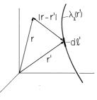
Fig. 4.5.4 An element of line charge at the position  $\mathbf{r}'$  gives rise to a potential at the observer location  $\mathbf{r}$ .
