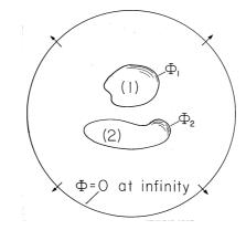
Fig. 4.6.2 Pair of electrodes used to define capacitance.
