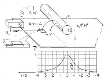
Fig. 4.7.2 Charge induced on ground plane by overhead conductor is measured by probe. Distribution shown is predicted by (4.7.7).
