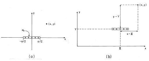
**Fig. 4.8.2** (a) Charge strip of Fig. 4.5.8 centered at origin. (b) Charge strip translated so that its center is at (X, Y).
