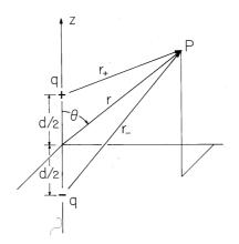
Fig. 4.4.1 Point charges of equal magnitude and opposite sign on the z axis.
