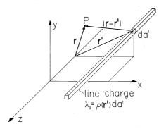
Fig. 4.5.7 For two-dimensional charge distributions, the elementary charge takes the form of a line charge of infinite length. The observer and source position vectors,  $\mathbf{r}$  and  $\mathbf{r}'$ , are two-dimensional vectors.
