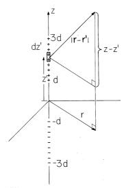
Fig. 4.5.5 Collinear positive and negative line elements of charge symmetrically located on the z axis.
