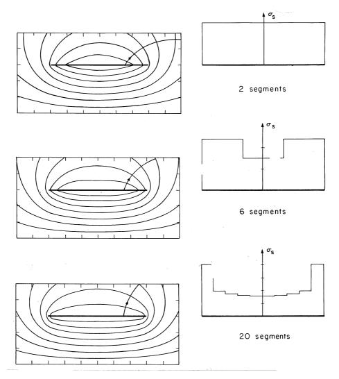
Fig. 4.8.4 Potential distributions using 2, 6, and 20 sheets to approximate the fields of a plane parallel capacitor. Only the fields in the upper half-plane are shown. The distributions of surface charge density on the upper plate are shown to the right.
