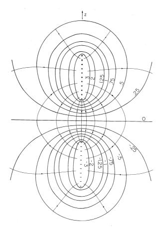
Fig. 4.5.6 Cross-section of equipotential surfaces and lines of electric field intensity for the configuration of Fig. 4.5.5.
