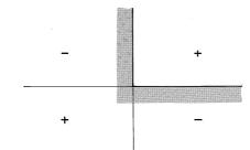
Fig. 4.7.3 Image charges arranged to satisfy equipotential conditions in two planes.
