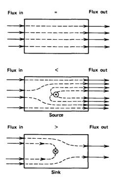
Figure 1-13 The net flux through a closed surface tells us whether there is a source or sink within an enclosed volume.
