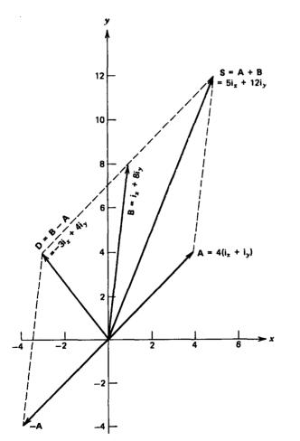
Figure 1-6 The sum and difference of vectors A and B given in Example 1-1.
