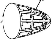
Figure 1-23 Many incremental line contours distributed over any surface, have nonzero contribution to the circulation only along those parts of the surface on the boundary contour L.
