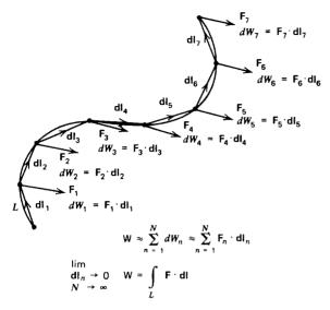
Figure 1-11 The total work in moving a body over a path is approximately equal to the sum of incremental works in moving the body each small incremental distance **dl**. As the differential distances approach zero length, the summation becomes a line integral and the result is exact.
