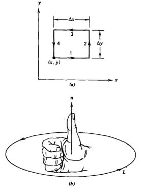
Figure 1-19 (a) Infinitesimal rectangular contour used to define the circulation. (b) The right-hand rule determines the positive direction perpendicular to a contour.
