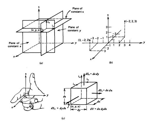
Figure 1-1 Cartesian coordinate system. (a) Intersection of three mutually perpendicular planes defines the Cartesian coordinates (x, y, z). (b) A point is located in space by specifying its x-, y- and z-directed distances from the origin. (c) Differential volume and surface area elements.
