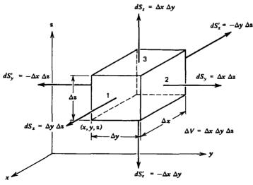
Figure 1-15 Infinitesimal rectangular volume used to define the divergence of a vector.
