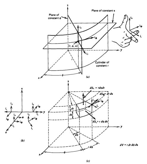
Figure 1-2 Circular cylindrical coordinate system. (a) Intersection of planes of constant z and  $\phi$  with a cylinder of constant radius r defines the coordinates (r,  $\phi$ , z). (b) The direction of the unit vectors  $\mathbf{i}_r$  and  $\mathbf{i}_{\phi}$  vary with the angle  $\phi$ . (c) Differential volume and surface area elements.
