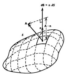
Figure 1-14 The flux of a vector  $\mathbf{A}$  through the closed surface S is given by the surface integral of the component of  $\mathbf{A}$  perpendicular to the surface S. The differential vector surface area element  $\mathbf{dS}$  is in the direction of the unit normal  $\mathbf{n}$ .
