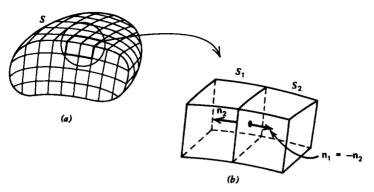
Figure 1-17 Nonzero contributions to the flux of a vector are only obtained across those surfaces that bound the outside of a volume. (a) Within the volume the flux leaving one incremental volume just enters the adjacent volume where (b) the outgoing normals to the common surface separating the volumes are in opposite directions.
