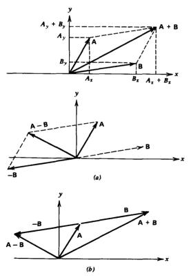
Figure 1-5 The sum and difference of two vectors (a) by finding the diagonal of the parallelogram formed by the two vectors, and (b) by placing the tail of a vector at the head of the other.
