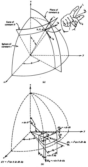
Figure 1-3 Spherical coordinate system. (a) Intersection of plane of constant angle  $\phi$  with cone of constant angle  $\theta$  and sphere of constant radius r defines the coordinates  $(r, \theta, \phi)$ . (b) Differential volume and surface area elements.
