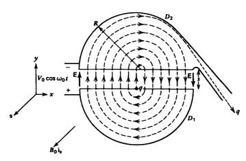
Figure 5-5 The cyclotron brings ions to high speed by many small repeated accelerations by the electric field in the gap between dees. Within the dees the electric field is negligible so that the ions move in increasingly larger circular orbits due to an applied magnetic field perpendicular to their motion.
