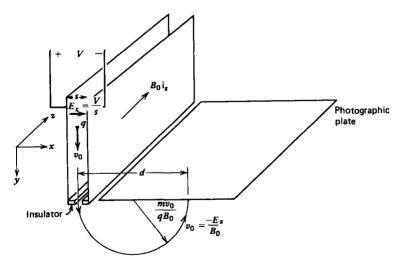
Figure 5-4 The mass spectrograph measures the mass of an ion by the radius of its trajectory when moving perpendicular to a magnetic field. The crossed uniform electric field selects the ion velocity that can pass through the slit.
