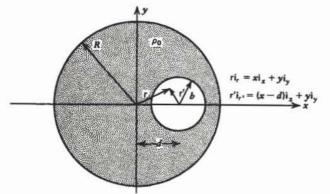
26. An infinitely long cylinder of radius R with uniform volume charge density  $\rho_0$  has an off-axis hole of radius b with center a distance d away from the center of the cylinder.
