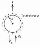
A spherical droplet of radius R and effective mass density  $\rho_m$  carries a total charge q in a gravity field g. What electric field  $E_0 \mathbf{i}_x$  will suspend the charged droplet? Millikan found by this method that all droplets carried integer multiples of negative charge  $e = -1.6 \times 10^{-19}$  coul.
