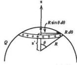
(a) Break the spherical surface into hoops of line charge of thickness  $R d\theta$ . What is the radius of the hoop, its height z', and its total incremental charge dq?
