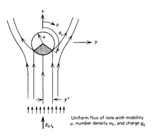
(a) If the uniformly distributed charge per unit length on the cylinder is  $\lambda(t)$ , what is the field distribution? Where is the electric field zero? This point is called a critical point because ions flowing past one side of this point miss the cylinder while those on the other side are collected. What equation do the field lines obey? (**Hint:** To the field solution of Section 4-3-2*a*, add the field due to a line charge  $\lambda$ .)
