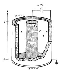
(a) What are the potential and electric field distributions within the structure (a < r < c, 0 < z < l)? (Hint: Try the zero separation constant solutions n = 0, k = 0.)
