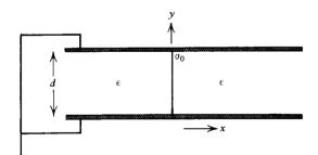
(a) What are the potential and electric field distributions? (**Hint:** Write  $\sigma_0$  as a Fourier series.)
