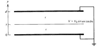
(a) What are the potential and electric field distributions? (**Hint:** You can write the potential distribution by inspection using a spatially shifted hyperbolic function  $\sinh c(y-d)$ .)
