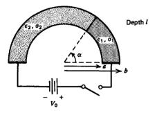
(a) What are the potential and electric field distributions within the shell at times t = 0,  $t = \infty$ , and during the transient interval? (Hint: Assume potentials of the form  $V(\phi) = A(t)\phi + B(t)$  and neglect effects of the region outside the half cylindrical shell.)
