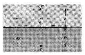
(a) Find the image currents I' at position x = -d and I'' at x = d that satisfy all the boundary conditions. The field in region 1 is due to I and I' while the field in region 2 is due to I''. (Hint: See the analogous dielectric problem in Section 3-3-3.)
