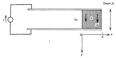
(a) Neglecting fringing field effects assume the magnetic field is  $H_z(x)\mathbf{i}_z$ . If the current is uniformly distributed throughout the slab, find the magnetic field everywhere.
