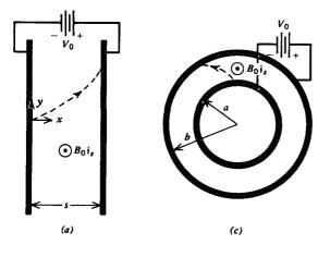
(c) A magnetron is built with coaxial electrodes where electrons are injected from r = a,  $\phi = 0$  with zero initial velocity. Using the relations from Table 1-2,
