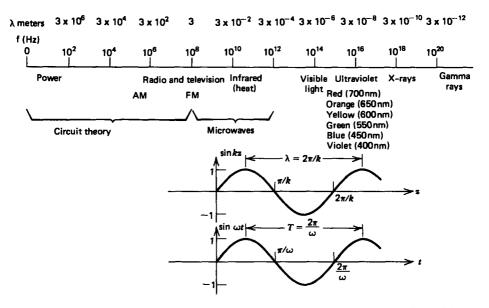
Figure 7-7 Time varying electromagnetic phenomena differ only in the scaling of time (frequency) and size (wavelength). In linear dielectric media the frequency and wavelength are related as  $f\lambda = c$  ( $\omega = kc$ ), where  $c = 1/\sqrt{\varepsilon\mu}$  is the speed of light in the medium.
