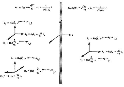
Figure 7-14 A uniform plane wave normally incident upon a dielectric interface separating two different materials has part of its power reflected and part transmitted.
