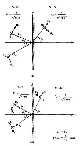
Figure 7-18 A uniform plane wave obliquely incident upon a dielectric interface also has its angle of incidence equal to the angle of reflection while the transmitted angle is given by Snell's law. (a) Electric field polarized parallel to the interface. (b) Magnetic field parallel to the interface.
