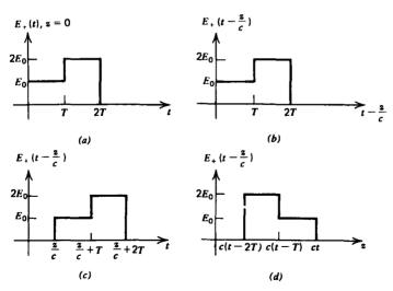
Figure 7-3 (a)  $E_+(t)$  at z=0 is a staircase pulse. (b)  $E_+(\phi)$  always has the same shape as (a) when plotted versus  $\phi$ , no matter what  $\phi$  is. Here  $\phi=t-z/c$ . (c) When plotted versus t, the pulse is translated in time where z must be positive to keep t positive. (d) When plotted versus z, it is translated and inverted. The pulse propagates at speed c in the positive z direction.
