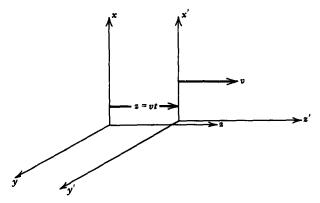
Figure 7-6 The primed coordinate system moves at constant velocity  $v_i$ , with respect to a stationary coordinate system. The free space speed of an electromagnetic wave is  $c_0$  as measured by observers in either coordinate system no matter the velocity v.
