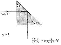
Figure 7-25 A totally reflecting prism. The index of refraction n must exceed  $\sqrt{2}$  so that the light incident on the hypotenuse at 45° exceeds the critical angle.
