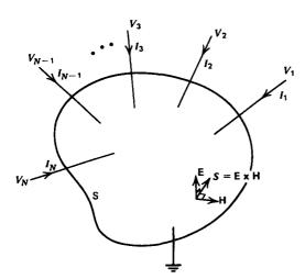
Figure 7-2 The circuit power into an N terminal network  $\sum_{k=1}^{N} V_k I_k$  equals the electromagnetic power flow into the surface surrounding the network,  $-\oint_S \mathbf{E} \times \mathbf{H} \cdot \mathbf{dS}$ .
