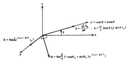
Figure 7-16 The spatial dependence of a uniform plane wave at an arbitrary angle  $\theta$  can be expressed in terms of a vector wavenumber  $\mathbf{k}$  as  $\mathbf{e}^{-j\mathbf{k}\cdot\mathbf{r}}$ , where  $\mathbf{k}$  is in the direction of power flow and has magnitude  $\omega/c$ .
