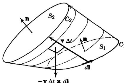
**Fig. B.4.2** When  $t = t$ , the surface  $S$  enclosed by the contour  $C$  is as indicated by  $S_1$  and  $C_1$ . By the time  $t = t + \Delta t$  this surface has moved to  $S_2$ , where it is enclosed by the contour  $C_2$ .
