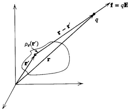
**Fig. B.1.1** The force  $\mathbf{f}$  on the point charge  $q$  in the vicinity of charges with density  $\rho_e(\mathbf{r}')$  is represented by the electric field intensity  $\mathbf{E}$  times  $q$ , where  $\mathbf{E}$  is found from (B.1.2).
