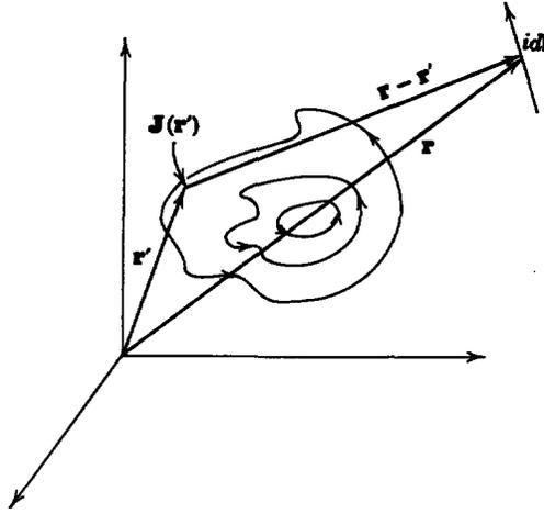
**Fig. B.1.4** A distribution of current density  $\mathbf{J}(\mathbf{r}')$  produces a force on the current element  $i d\mathbf{l}$  which is represented in terms of the magnetic flux density  $\mathbf{B}$  by (B.1.27) and (B.1.28).
