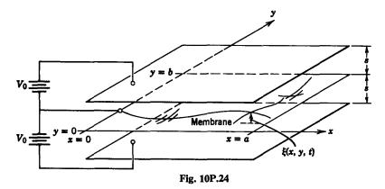
10.24. A perfectly conducting membrane with tension S and mass/unit area  $\sigma_m$  is fixed at x = 0 and x = a and at y = 0 and y = b. Perfectly conducting plane-parallel electrodes have an equilibrium distance s from the membrane and a potential  $V_0$  relative to the membrane.
