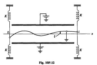
10.12. The conducting wire shown in Fig. 10P.12 is stressed by a transverse electric field and hence has transverse displacements that satisfy the force equation:
