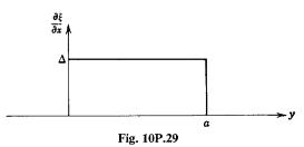
10.29. A membrane has the velocity  $U > v_s$  in the x-direction, as described in Section 10.4.2. At x = 0,  $\xi = 0$ , and  $\partial \xi / \partial x$  has the distribution shown.
