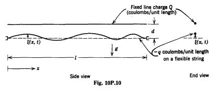
10P.10. This string, which has a tension f and mass per unit length m, supports a charge per unit length -q, where  $q \ll Q$  and both Q and q are positive.
