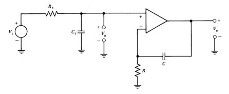
Figure 1.5 Noninverting integrator.
