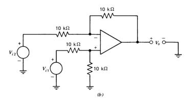
Figure 1.7 Differential-amplifier connections.
