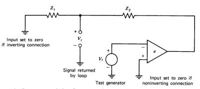
Figure 1.3 Loop transmission for connections of Fig. 1.2. Loop transmission is  $V_r/V_t = -a Z_1/(Z_1 + Z_2)$ .
