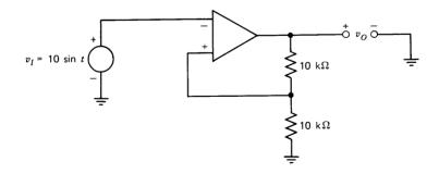
Figure 1.12 Schmitt trigger.
