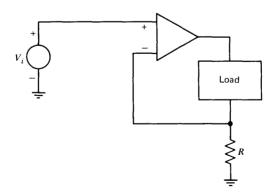
Figure 1.9 Circuit with controlled output resistance.
