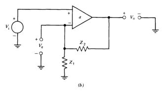
Figure 1.2 Operational-amplifier connections. (a) Inverting. (b) Noninverting.
