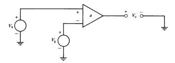
Figure 1.1 Symbol for an operational amplifier.
