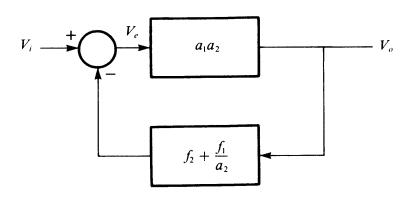
**Figure S1.4** Reduced block diagram.
