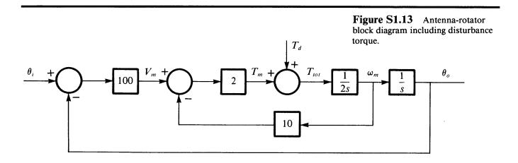
At this point, we save further calculations by using a diagram manipulation to move the  $T_d$  input to the same summing junction as  $\theta_i$ , yielding Figure S1.14:
