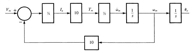
Lastly, we add the differential amplifier. With the error signal defined as in Figure 2.27, and an amplifier gain of 10, we have
