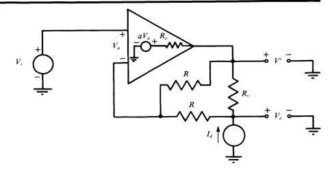
Because  $R \gg R_s$ , we assume that all of  $I_d$  flows through the series connection of  $R_o$  and  $R_s$ . Thus
