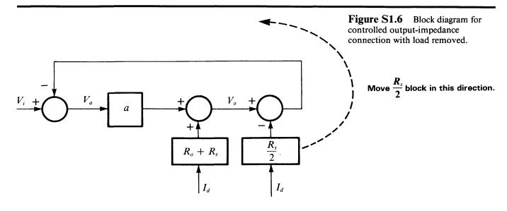
To calculate output-resistance  $R_{\rm amp}$ , we need the ratio  $\frac{V_o}{I_d}$ . Note that  $V_i$  does not affect this ratio (as a consequence of linearity); thus, we set  $V_i = 0$ . We then manipulate the block diagram by propagating the  $\frac{R_s}{2}$  block forward around the loop, as indicated in Figure S1.6, to arrive at the reduced block diagram of Figure S1.7:
